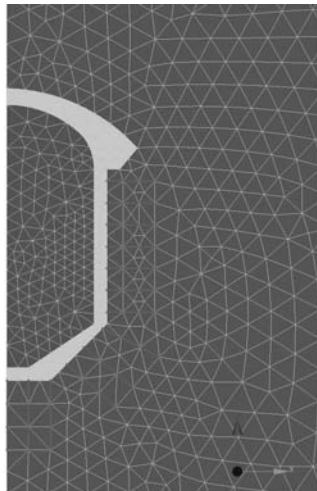
Fig.3. Finite element modelling of the underground settling Livezeni
